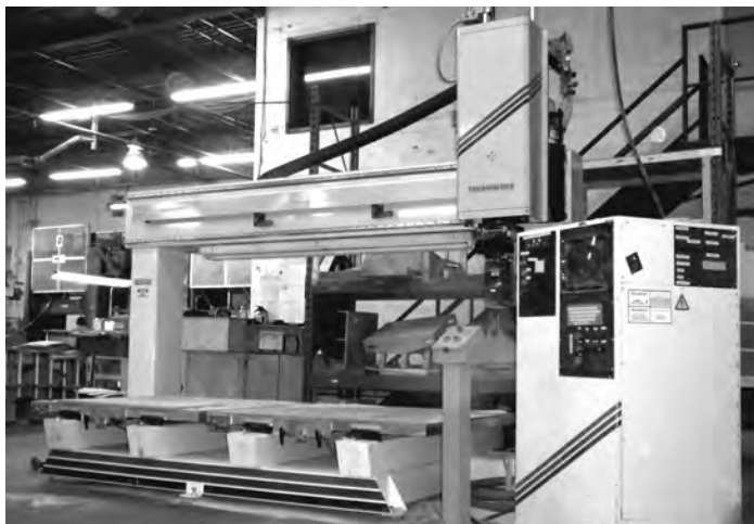
Thermwood 67 with 5-Axis CNC contour router
