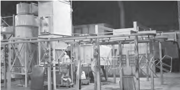
In-house Conveyorized Powder Coat application center
